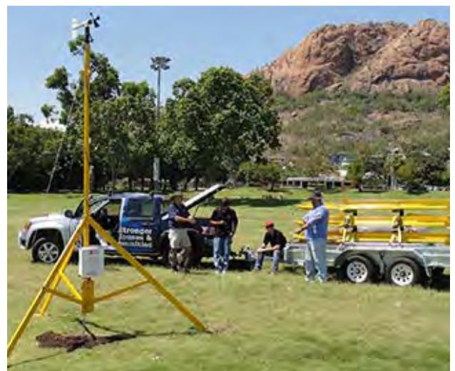
Image: Portable anemometer network for measuring wind speeds of tropical cyclones that impact the communities (courtesy: Cyclone Testing Station James Cook University)
