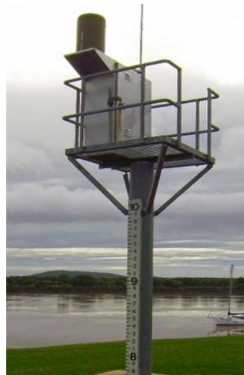
Automatic rain and river gauge with a manual read gauge for backup.
